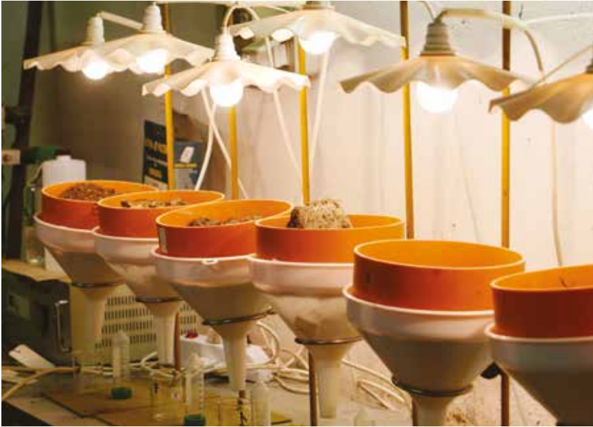
Microarthropods extraction by modified Berlese-Tullgren funnels.
