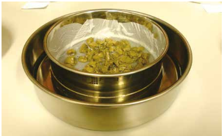
Soil nematode sampling by corer and nematode extraction by modified Baermann method.
